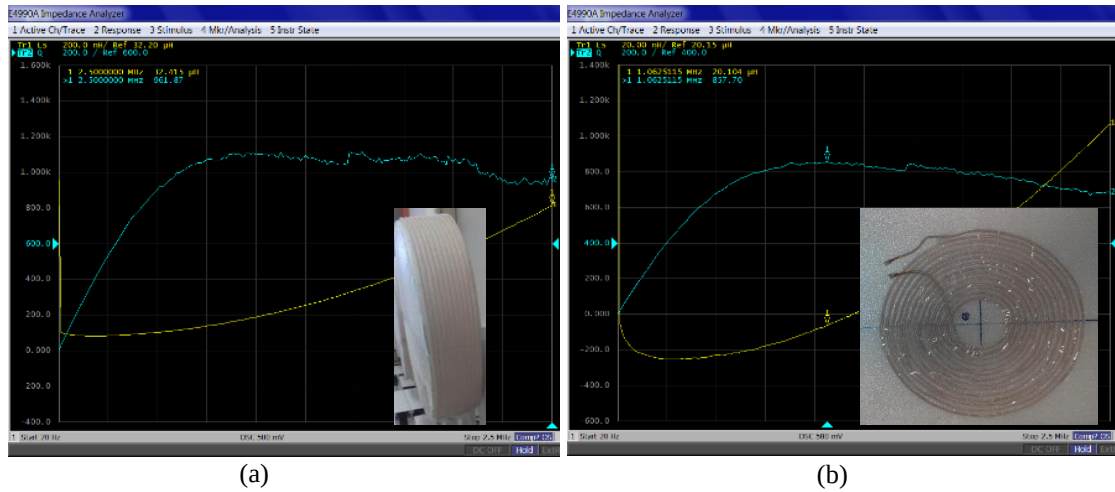
Fig. 3-19 Experimental quality factor characteristics (a) – Helical, (b) – Spiral
