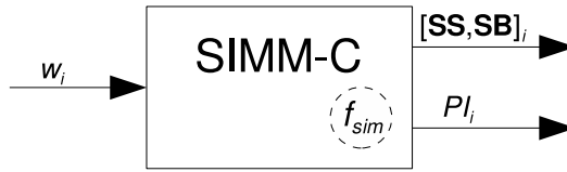
Figure 4.5: The simulation management component (SIMM-C) is using f_{sim} to simulate a what-if scenario w_i . Depending on the class of symbiotic simulation system (i.e., class A or class B/C) and the application-specific simulation engine, simulation results are either provided as state and behaviour information [\mathbf{SS}, \mathbf{SB}]_i or performance indicator information PI_i .
