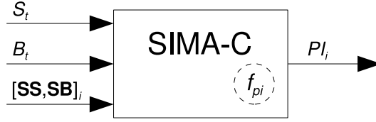
Figure 4.6: The simulation analysis component (SIMA-C) analyses simulation results [\mathbf{SS}, \mathbf{SB}]_i using f_{pi} and determines corresponding performance indicator values PI_i . Depending on the class of symbiotic simulation system, this may also involve using state and behaviour information ( S_t and B_t , respectively) from the physical system.
