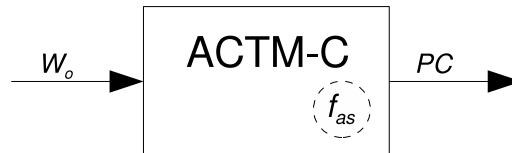
Figure 4.7: The action management component (ACTM-C) selects a what-if scenario from W_o using f_{as} and extracts the corresponding PC parameter values.
