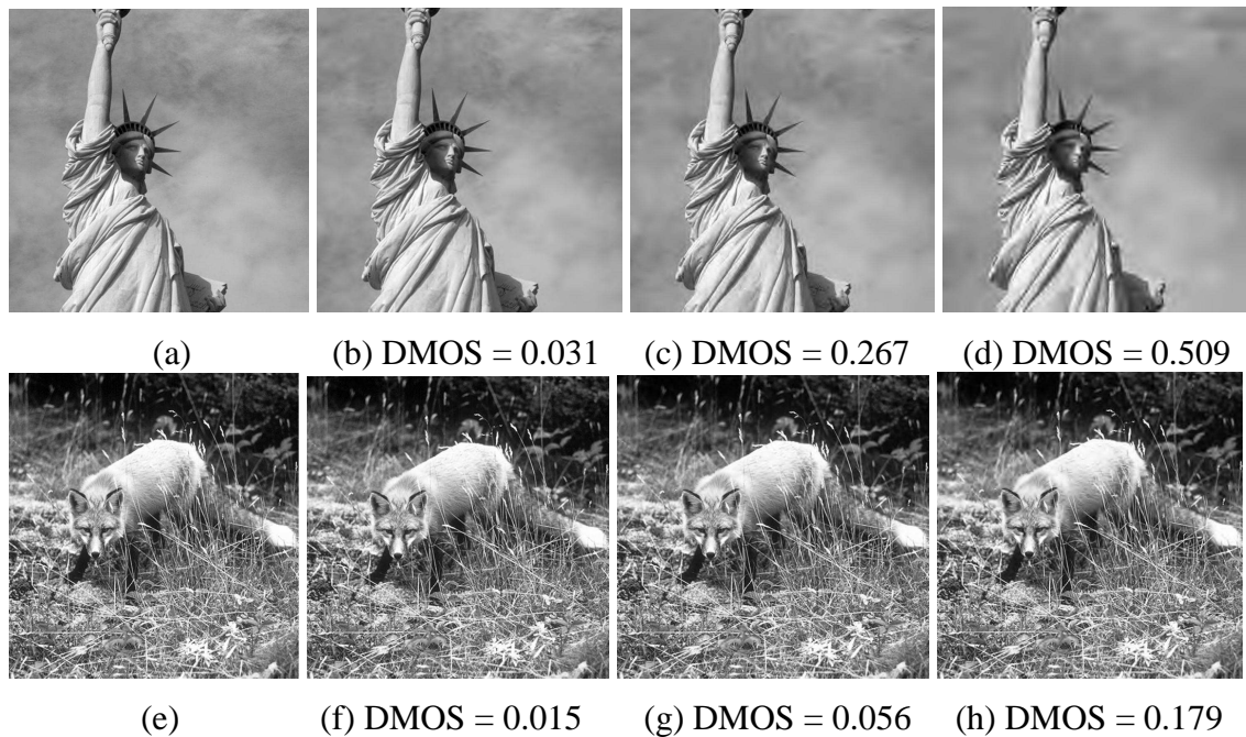
Figure 6.4: Effect of distortion on image with relatively more smooth areas and more textured areas (these images are from CSIQ image database).
