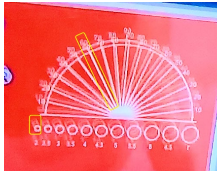
Figure 4.9 Visual analysis of the amplitude and lead angle based on the Vibroscope
