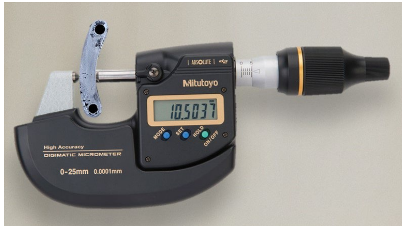
Figure 3.18 Mitutoyo Digital Ball Micrometre to measure thickness of airfoil
