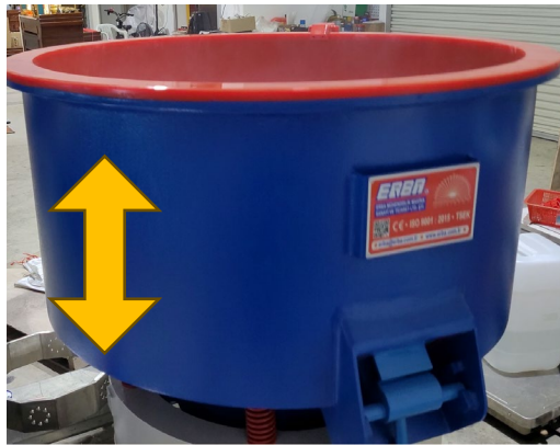
Figure 4.7 Domeless Bowl movement in the 90° lead angle due to the lack of eccentric mass to tilt the vibration
