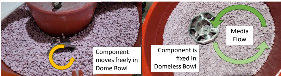
Figure 3.41 Free vs fixed fixturing between dome and domeless vibrofinishing process
