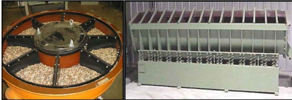
Figure 2.4 Compartmentalised Vibratory (left) bowl and (right) trough [16]
