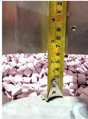
Figure 3.12 (a) Media Entry Height (labelled as H_{\text{Entry}} ) can be measured by subtracting (b) measured from component top surface to media surface on pre-process
