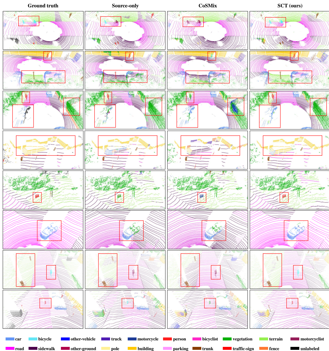
FIGURE 4.10: Qualitative comparison of SCT with the Source-only (with no adaptation) and the state-of-the-art CoSMix [4] in domain adaptive 3D LiDAR semantic segmentation. The comparison was conducted over the task “SynLiDAR → SemanticKITTI”. The ‘Ground truth’ denotes the ground-truth annotations. The red rectangles highlight regions of interest. Best viewed in color.
