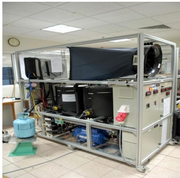
Figure 73 Picture of the lab scale vapor compression refrigeration system
