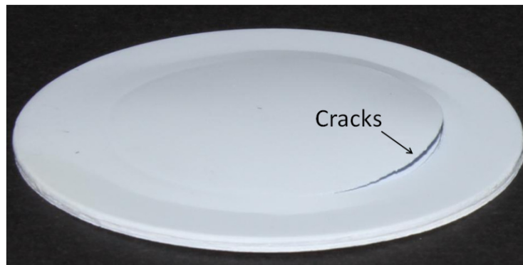
Figure 5-7 HL2000 embedded carbon sample after sintering at 10 K/min showing obvious cracks at edges of embedded cavity. No cross-sectioning was done as the defect is obvious.
