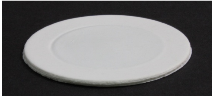
Figure 5-17 Embedded sample of composite layer of Ferro A6M/Dupont 951 firing at multi-step profile.
