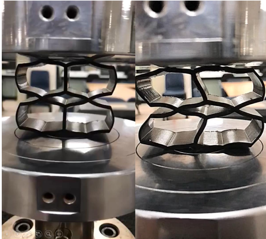
Figure 4-20: No deformation on vertical cell walls (Linear Phase); Buckling of inner vertical cell walls (Plateau Phase).
