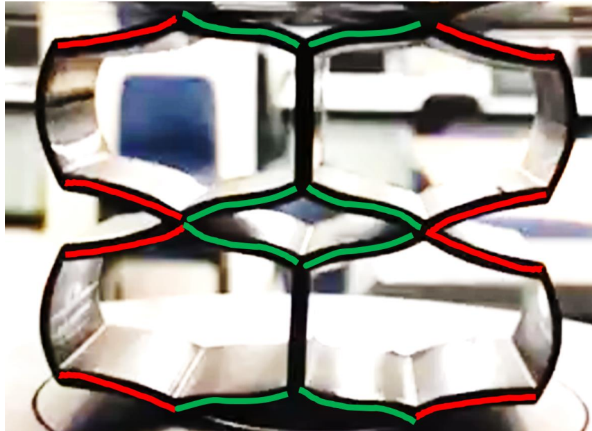
Figure 4-19: Half wave and full wave bending modes of the outer and inner cell walls respectively.
