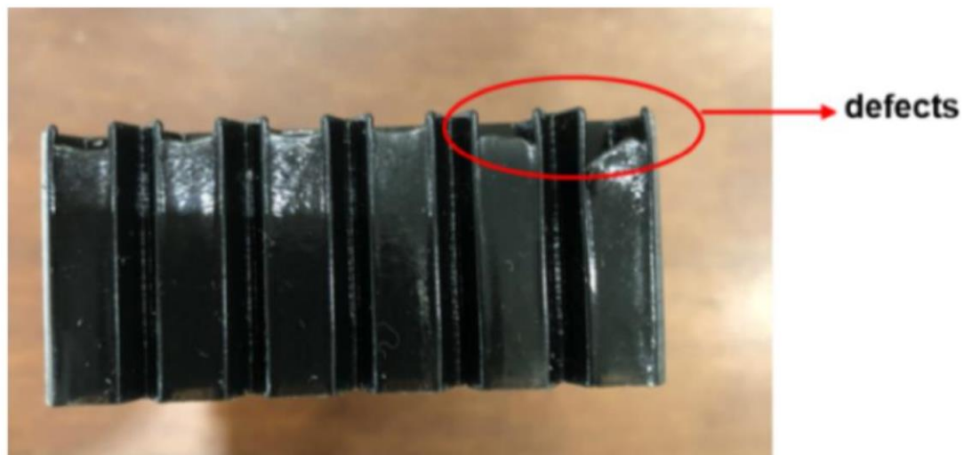
Figure 3-8: Incomplete building of thin walls during Polyjet printing process
