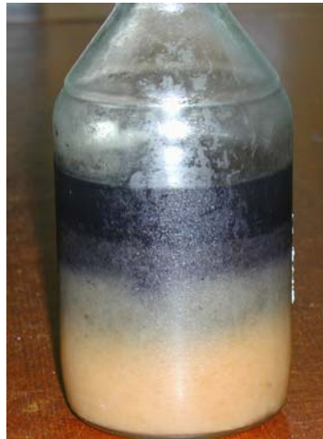
Fig.7-1 Appearance of PA-degrading aerobic granules after 8-week storage.
