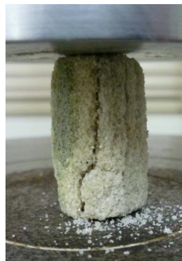
Figure 5.30 Typical UC specimen and its failure mode trimming from the water pond
