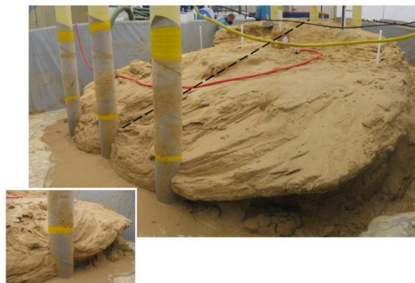
Figure 2.27 Remaining of the sand body (≈40m 3 ) after treatment (van Paassen et al, 2010)
