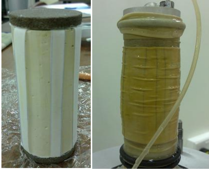
Figure 8.4 Images of specimen 2a: a) before conducting CID test, and b) after failure
