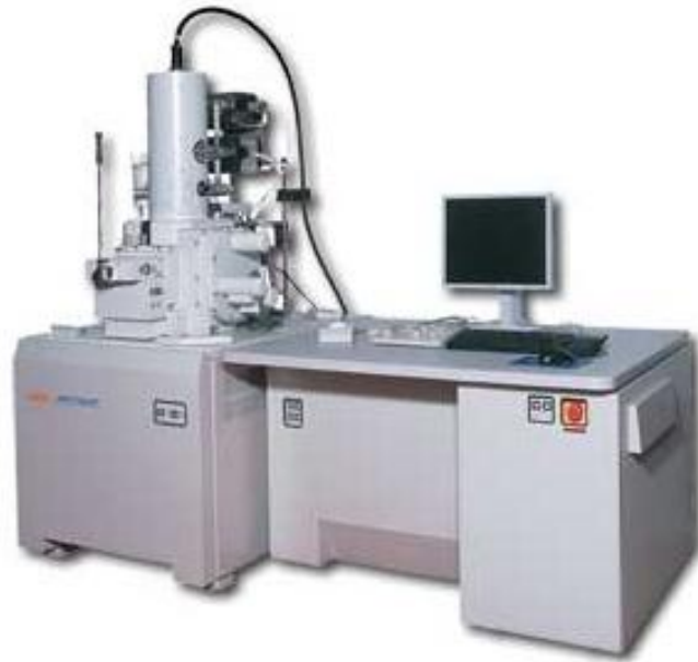
Figure 3.12 Image of field emission scanning electron microscope (FE-SEM) with energy dispersive X-ray spectroscopy (EDS) employed in this study
