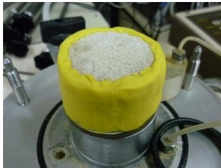
Figure 3.9 Image of a typical specimen prepared for flexible wall permeability test in triaxial apparatus
