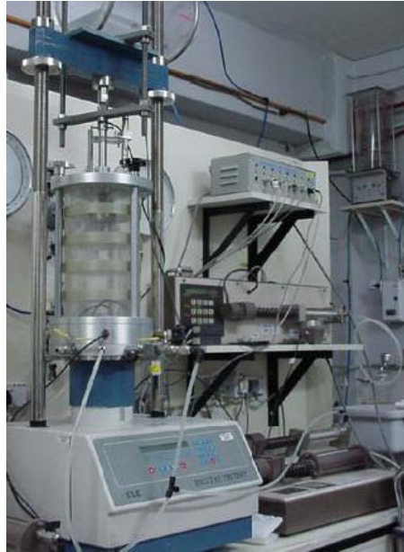
Figure 3.6 Overview of triaxial test apparatus.
