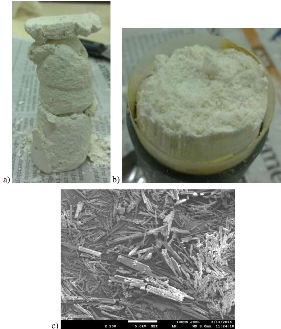
Figure 8.16 Figure of kaolin specimens at zero water content: a) mixing with 3M urea; b) urea crystal leaching from specimen's surface; c) SEM picture of the urea crystal in b)
