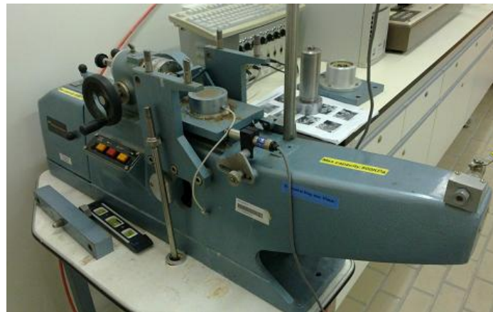
Figure 3.10 Schematic and image of direct simple shear apparatus setup (after Meng, 2010)
