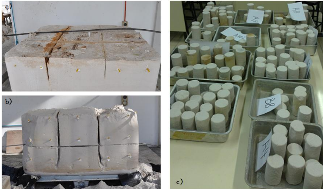
Figure 6.6 Images of the cubic meter biotreated sand box during: a) cutting of the first layer A; b) cutting of second and third layer B and C; c) part of the specimens drilled for strength and permeability test
