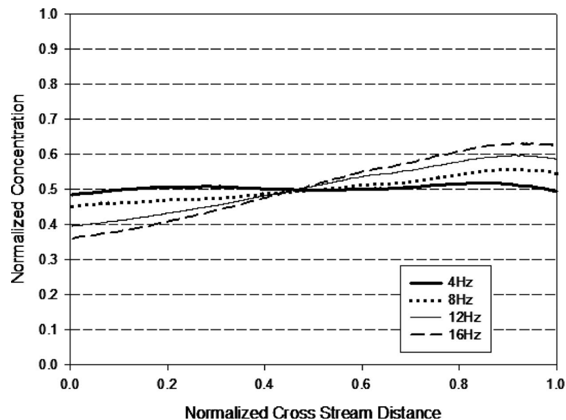
FIG. 17. Normalized concentration distribution across width of micromixer design D (at 1.2 mm after T-junction) with applied ac amplitude E_{ac}=4/3E_{dc} . Cross stream distance is normalized with width of channel ( 200 \mu\text{m} ).
