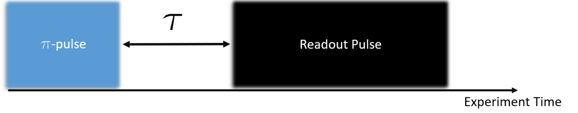
Figure 23: Pulse sequence of a T_1 experiment. A \pi -pulse and readout pulse is sent to the system and the delay \tau is varied between the two pulses.
