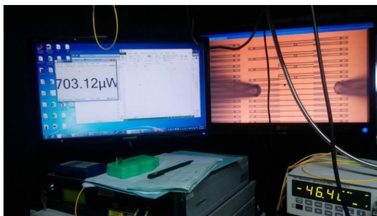
Fig.2.17 The alignment of the input fiber and the waveguide with grating coupler.
