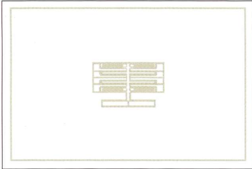
Figure 63: Mask 5 (comb finger features)
