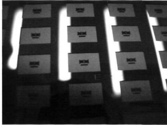
Figure 75: Structures formed after back etching (on silicon wafer)
