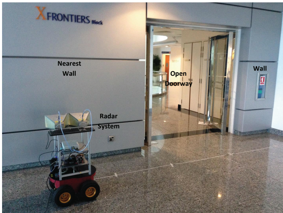
Figure 4.1: Doorway Detection Environment
