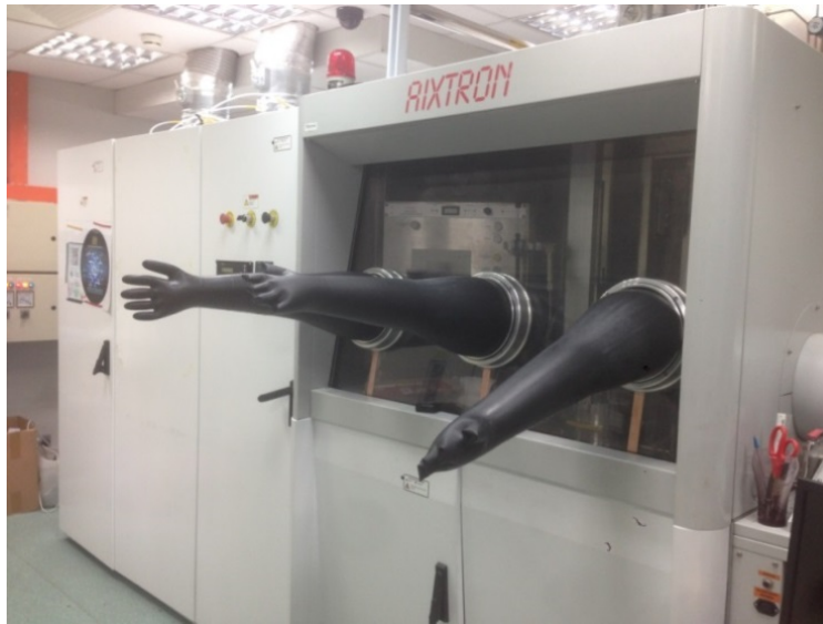
Figure. A1 Appearance of 3×2" AIXTRON CCS MOCVD system in our group.
