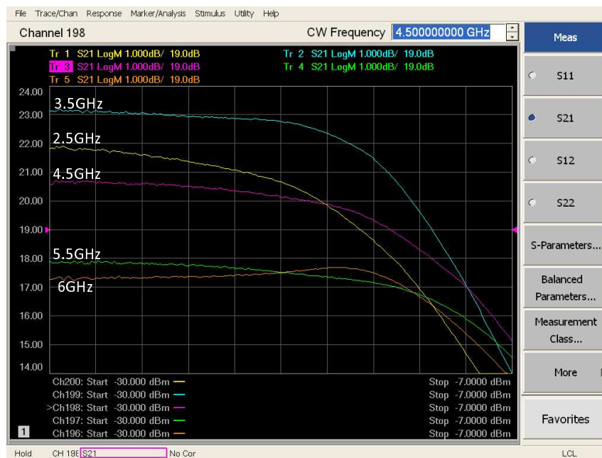
Figure 5.18: Measured large signal performance of dual-feed 3-stage DPA. Note: The response before externally added driver amplifier parameters are de-embedded.
