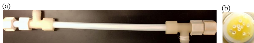
Fig. 3.1 Photographs of (a) fabricated membrane module; (b) cross section of the module.
