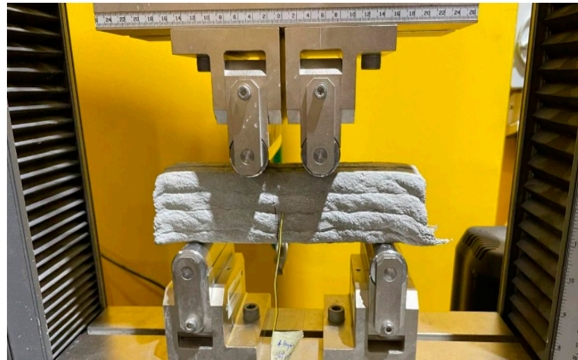
Figure 4. Four-point bending test setup.
