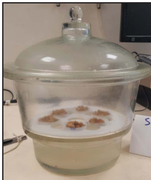
Figure 7: SWCC process by salt solution method
