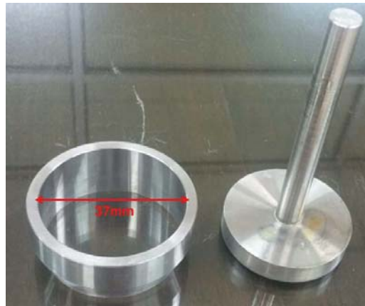
269 Figure 11. Specimen trimmer and pusher to prepare specimen for 270 dew-point chilled mirror device
