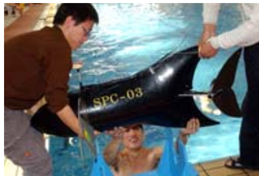
Figure 2.4. Robotic fish developed by BUAA and CAS of China. The technicians are sending the fish into the swimming pool for testing [15].
