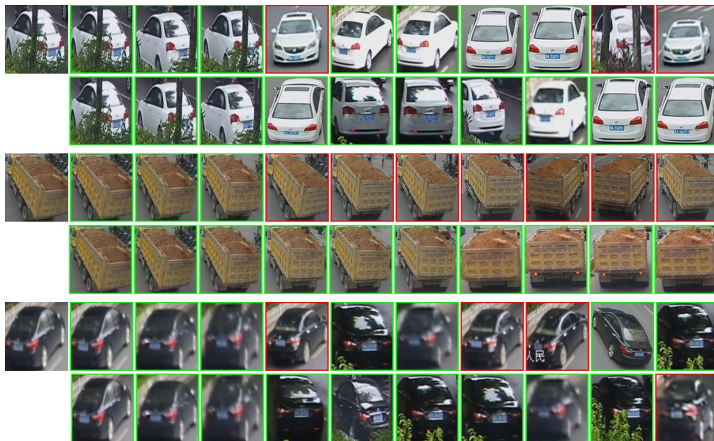
FIGURE 4.1: Visualization of vehicle Re-ID ranking list on VeRi776. The images on the first column are the query images and the rest show retrieved gallery images. For each query sample, the first and second row respectively shows the top-5 results by baseline and PMANet. we draw the correct and false matched vehicle images respectively with green and red rectangles.
