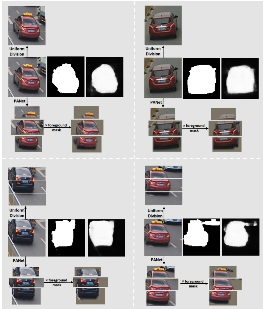
FIGURE 4.2: Examples of generated masks by Uniform Division and our PANet. The sub-figure on the first row illustrate three parts vertically split by Uniform Division. The three figures on the second row respectively represent the sample image, the coarse foreground mask by GrabCut [52] and the refined one by our PANet. On the third row, the two sub-figures exhibit the K different part masks predicted by PANet and these K part masks multiplied with the refined foreground mask.
