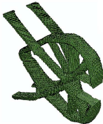
Figure 2.13: A compliant gripper synthesized by BESO method [59].
