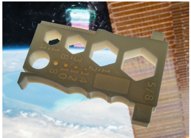
Fig. 4 The MPMT, created by a university student as part of the “Future Engineers Space Tool Challenge”, printed on the ISS [45].
