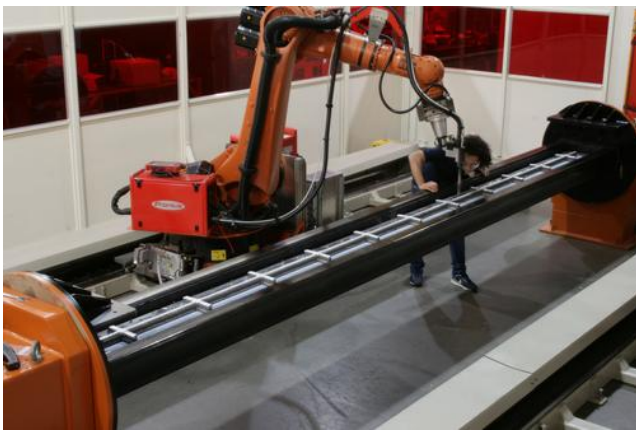
Fig. 19 Cranfield University’s WAAM 3D printer being used to print a double-sided, six metres long aluminium spar [139].
