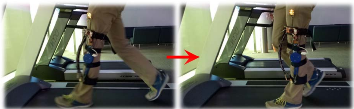
Figure 6. Testing of the integration system of supercapacitor and human motion energy harvester. The energy harvester powers the LED and charges the supercapacitor device with energy
