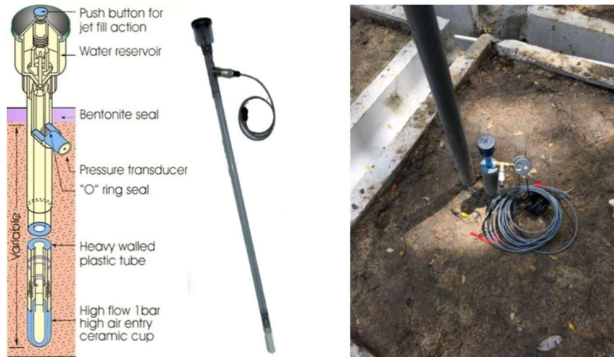
Figure 31: Jet-fill tensiometer with transducer used in this study
