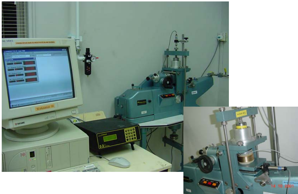
Figure 3.20 Set-up for DSS Testing System
