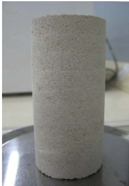
Figure 3.9 Artificially Cemented Soil Specimen for Triaxial Test
