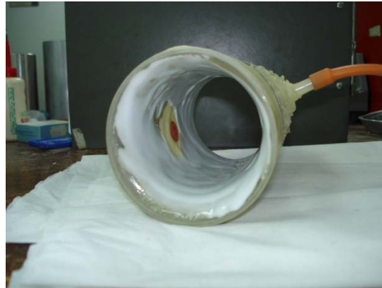
Figure 3.16 Liquid Rubber Applied inside Rubber Membrane
