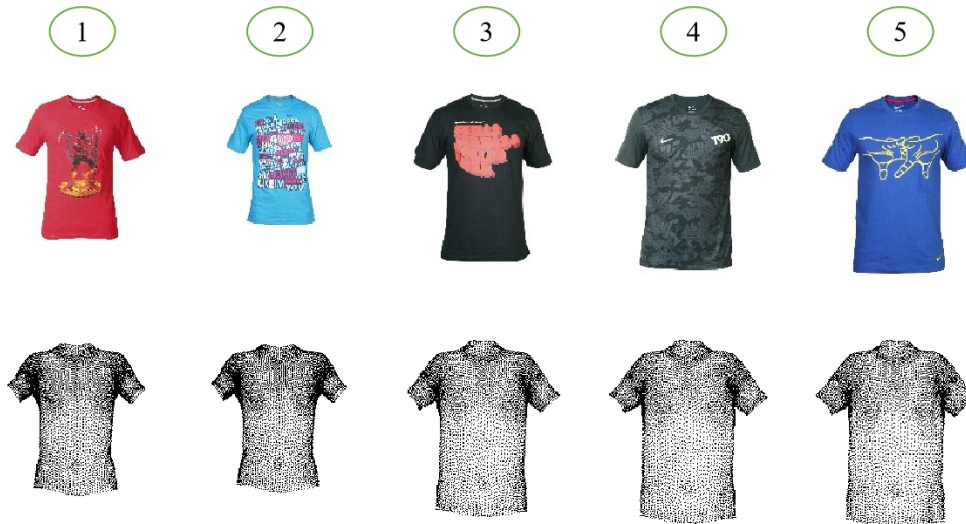
Figure 3.8: Overview of the test outputs of the network. The upper row is the input 2D RGB garment images which are split out from the dataset before training. The lower row is the corresponding projected 3D garment mesh vertices from the generated 3D garment meshes during testing.
