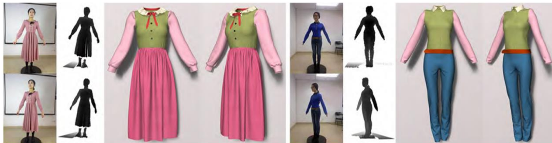
Figure 2.5: With RGBD sequence as input, the network [21] detects and assembles the suitable components to produce a high-quality 3D garment model
