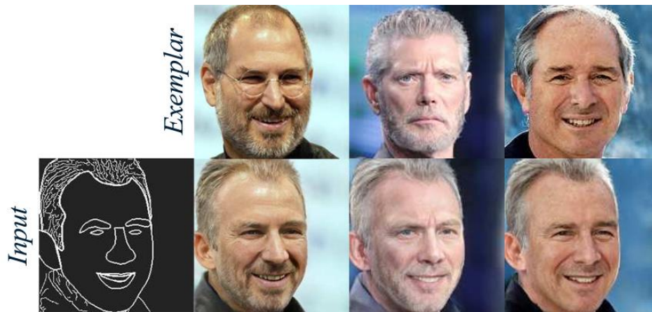
Figure 1.10: Exemplar-based image synthesis [96]. The 1 st row is the exemplar images and the second row is the synthesized images from the network
