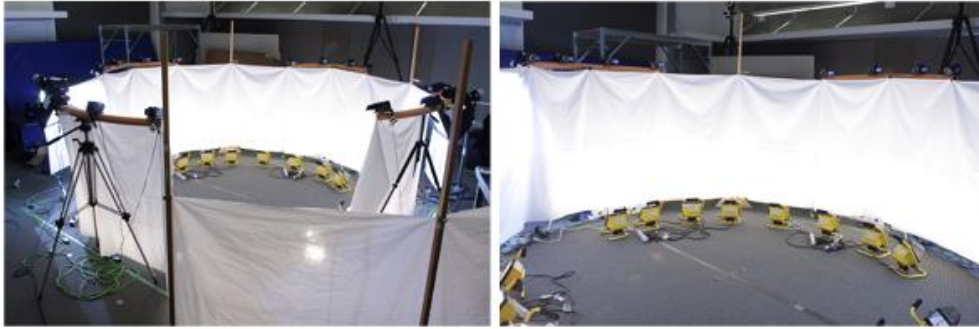
Figure 1.3: Acquisition setup for multi-view images [19]
