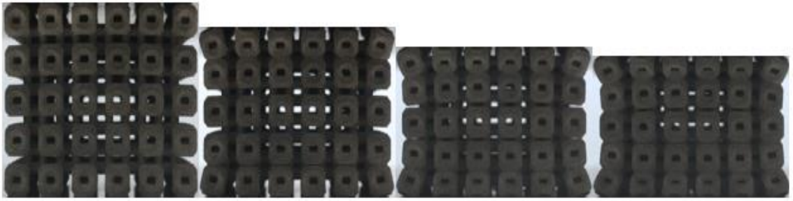
Figure 6.16. The optical images of the evolution of the deformation patterns for auxetic bcc-6H lattices with the relative densities of 0.3.
