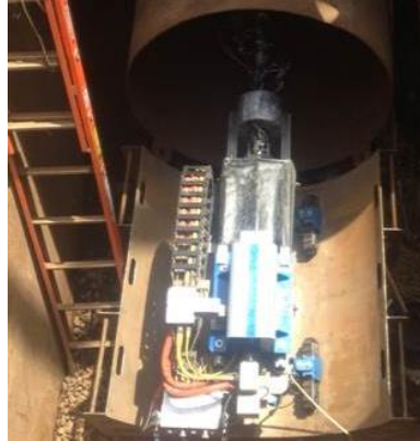
Figure 2.14: Quest Inspar's PipeArmor robot [19]
