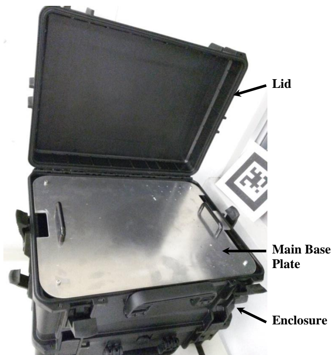
Figure 4.10: The main base plate for components mounting
