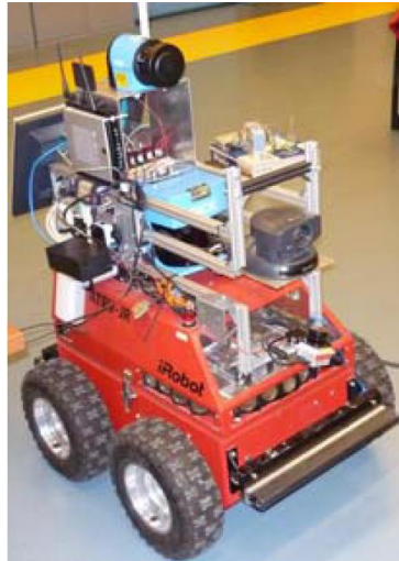
Figure 2.8: ATRV Jr with 3D sensors [11]
