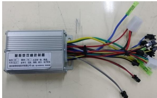
Figure 5.4: Hub Motor Controller
