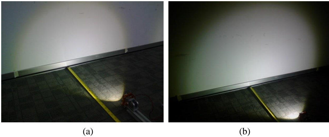
Figure 4.7: The beam angle of LED with (a) 80° lens and (b) 100° lens
