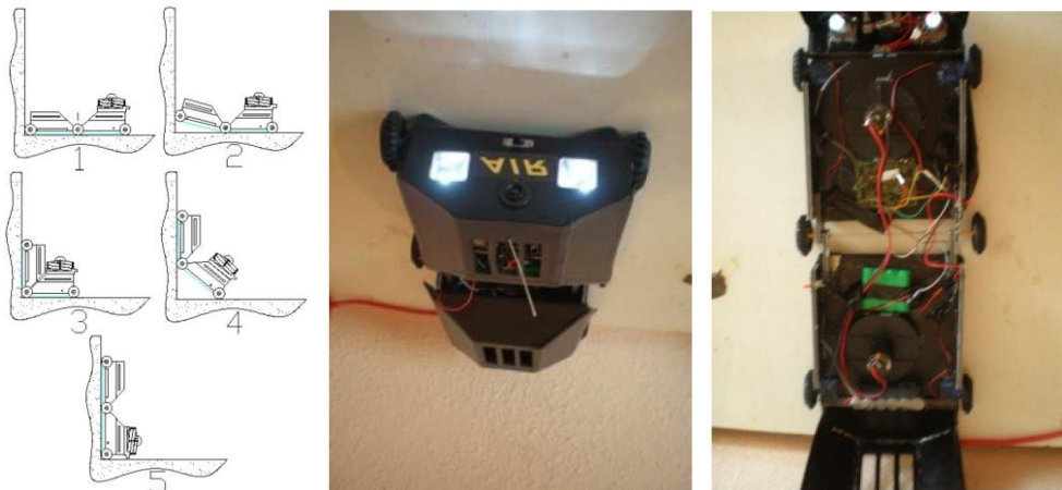
Figure 2.7: A modular pipe cleaning mobile equipment [10]
