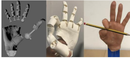
Fig. 3. Our robotic hand's 3D model and the final product
