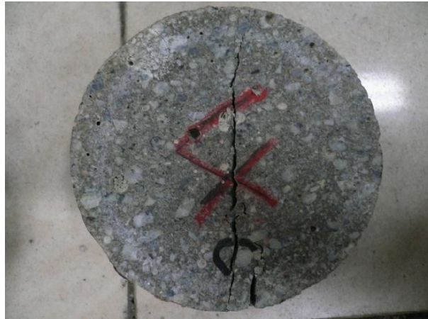
Figure 7.29 the specimen used in experimental Brazilian test after failure (Yu, Zhang et al. 2009)
