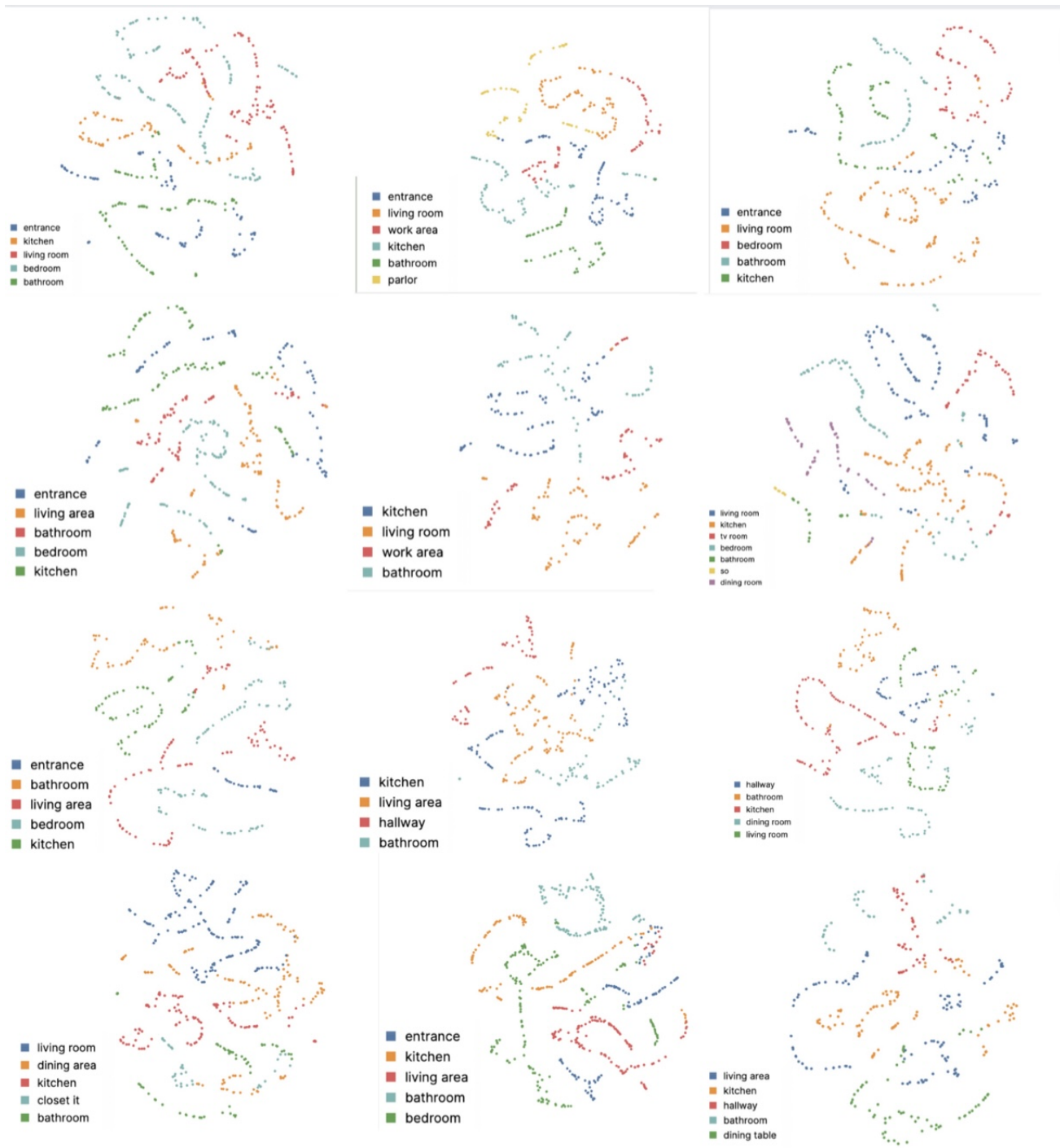
Figure 16: The participant house embedding maps (computed by Fig. 14) show home variability with no clear clusters, indicating that standard clustering or CNN room detection models are unsuitable. The map displays 2D image embeddings, color-coded by room after dimensionality reduction.
