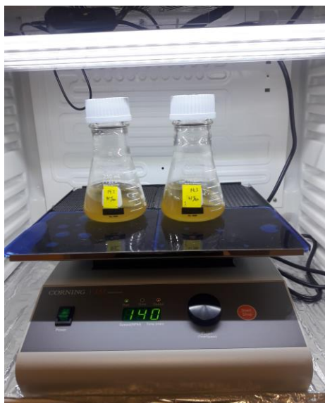
Figure 2. Microalgae culture setup in a chilling incubator with white fluorescence light and an orbital shaker.
