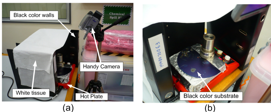
Figure 3.4: Setup of annealing experiments in laboratory, a) far view, b) close view.
