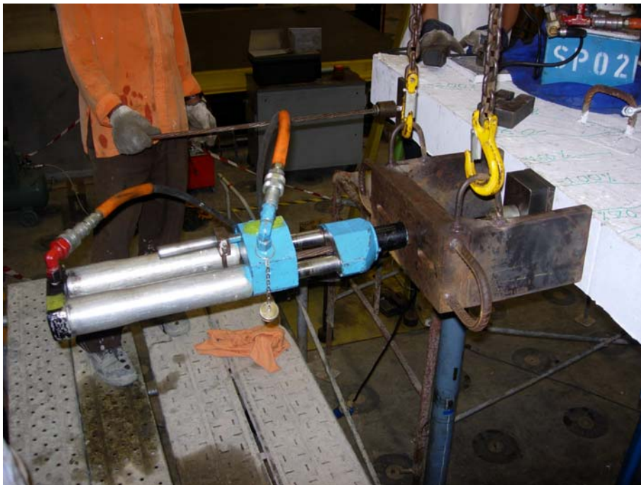
Fig. B.10 De-stressing of tendons
