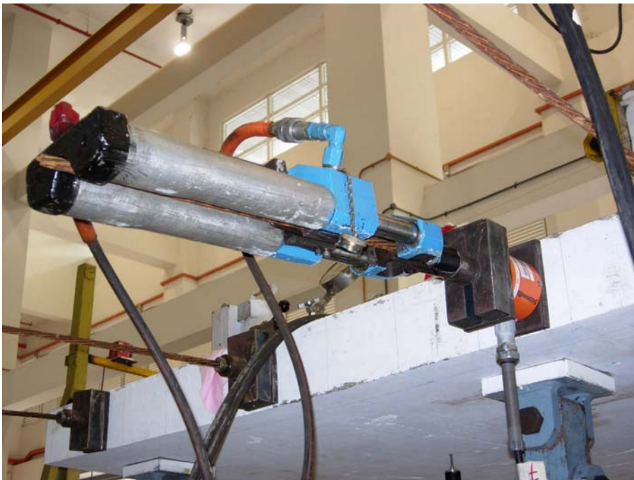
Fig. B.8 Stressing of tendon
