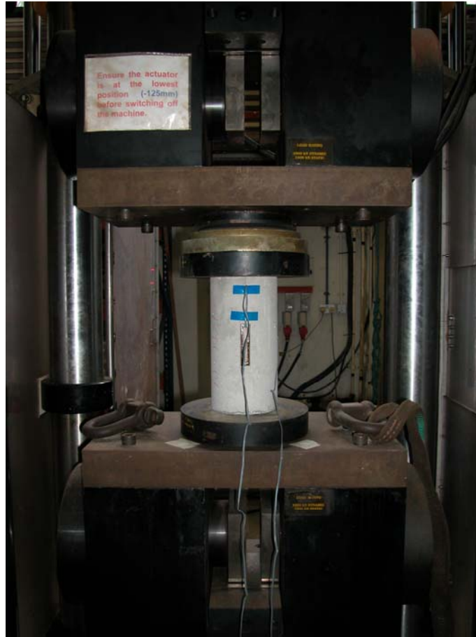
Fig. B.5 Compression test of concrete cylinders
