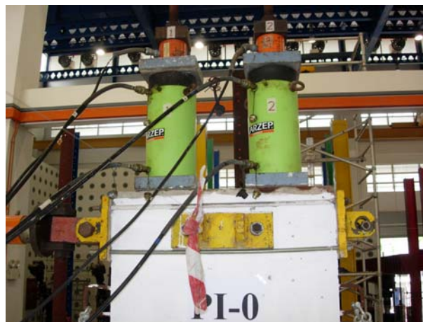
Figure 4.11 Prestressing rods with jacks
