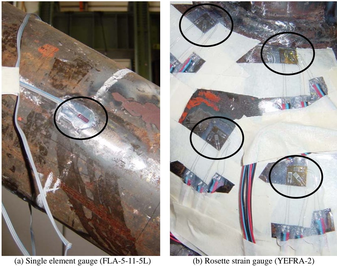
Fig. 3.10 Strain gauges on the test specimens
