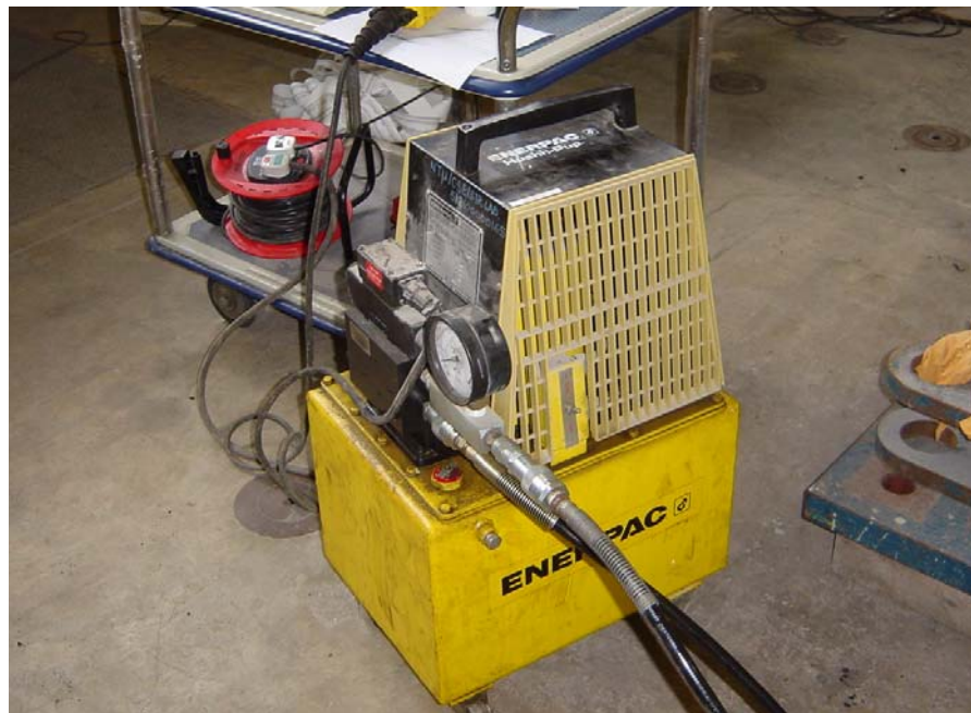
Fig. 3.7 Electrically operated pump used in the tests
