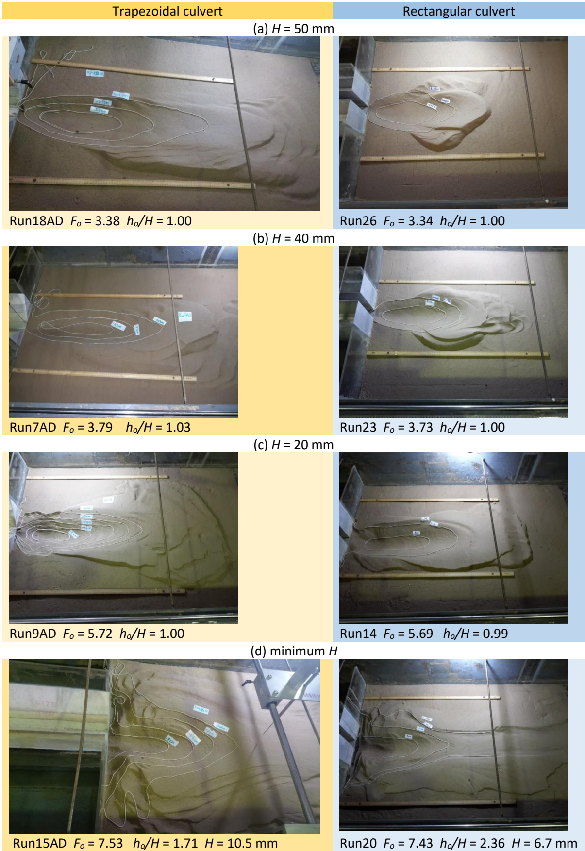
Figure 3.29 Photos from trapezoidal and rectangular culvert experiments showing the differences between the scour holes at similar tailwater depth.
