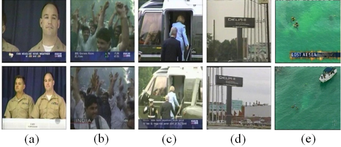
Figure 3.1: Challenging NDK examples — Examples of NDKs with zooming in (a) and (c), object/camera motion in (b) and (d), low number of keypoints in (e).
