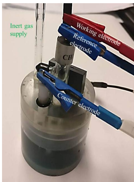
Figure 3.2. Electrochemical cell with three electrodes set up for CV and EIS measurements.
