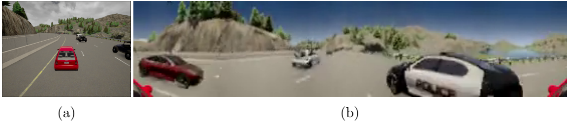
Fig. 4.12: (a) Illustration of a third-person view in ‘Town4’ scenario of CARLA. (b) A first-person observation for RL agent. It concatenates five cameras for 300 degrees view
