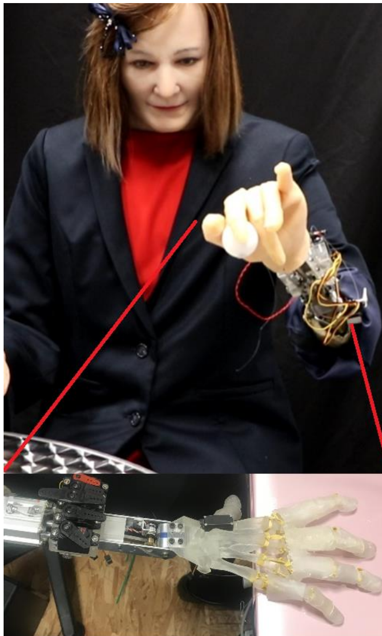
Figure 5-9 Installation with Nadine Robot. The servo bed is linked to the forearm frame of the robot
