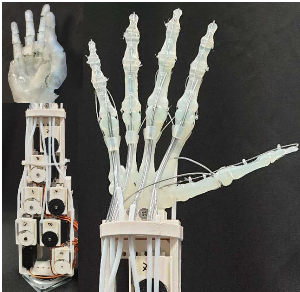
Figure 6-1 The robotic hand part consists of 4 materials: 3D printed bones, 3D printed elastic tissues, nylon cable and Bowden cable with pipes. Left top: Artificial tissue. Left down: servo bed with 13 servo motor
