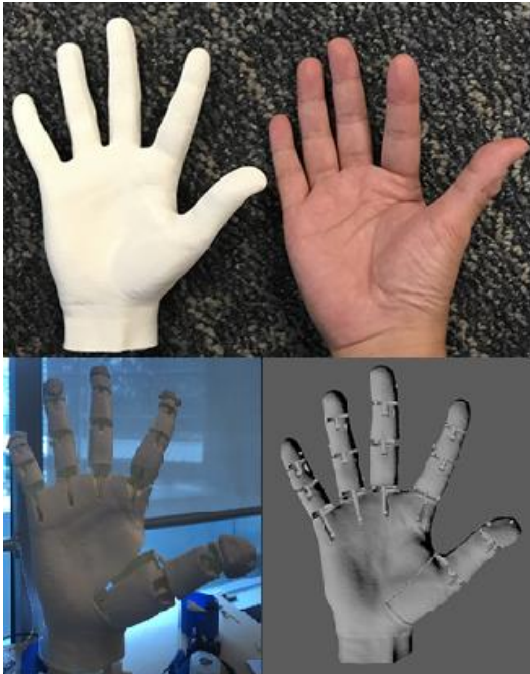
Figure 3-9 (Top) 3D-printed scanned hand and natural hand (Bottom) our robotic hand and its 3D model
