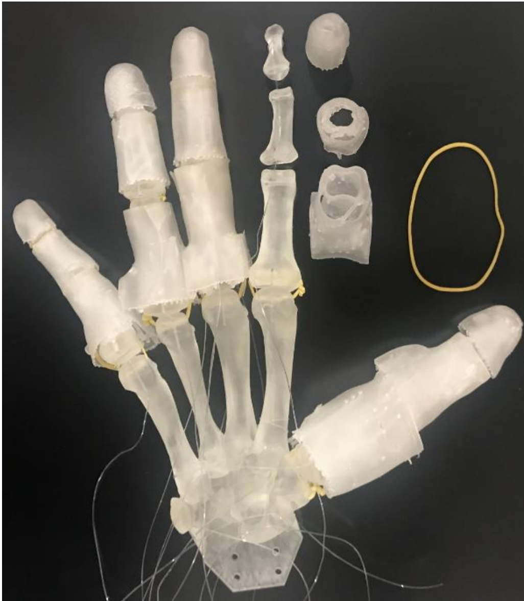
Figure 4-3 The proposed robotic hand consists of 4 materials: 3D printed bones, 3D printed elastic tissues, nylon cable and rubber band.
