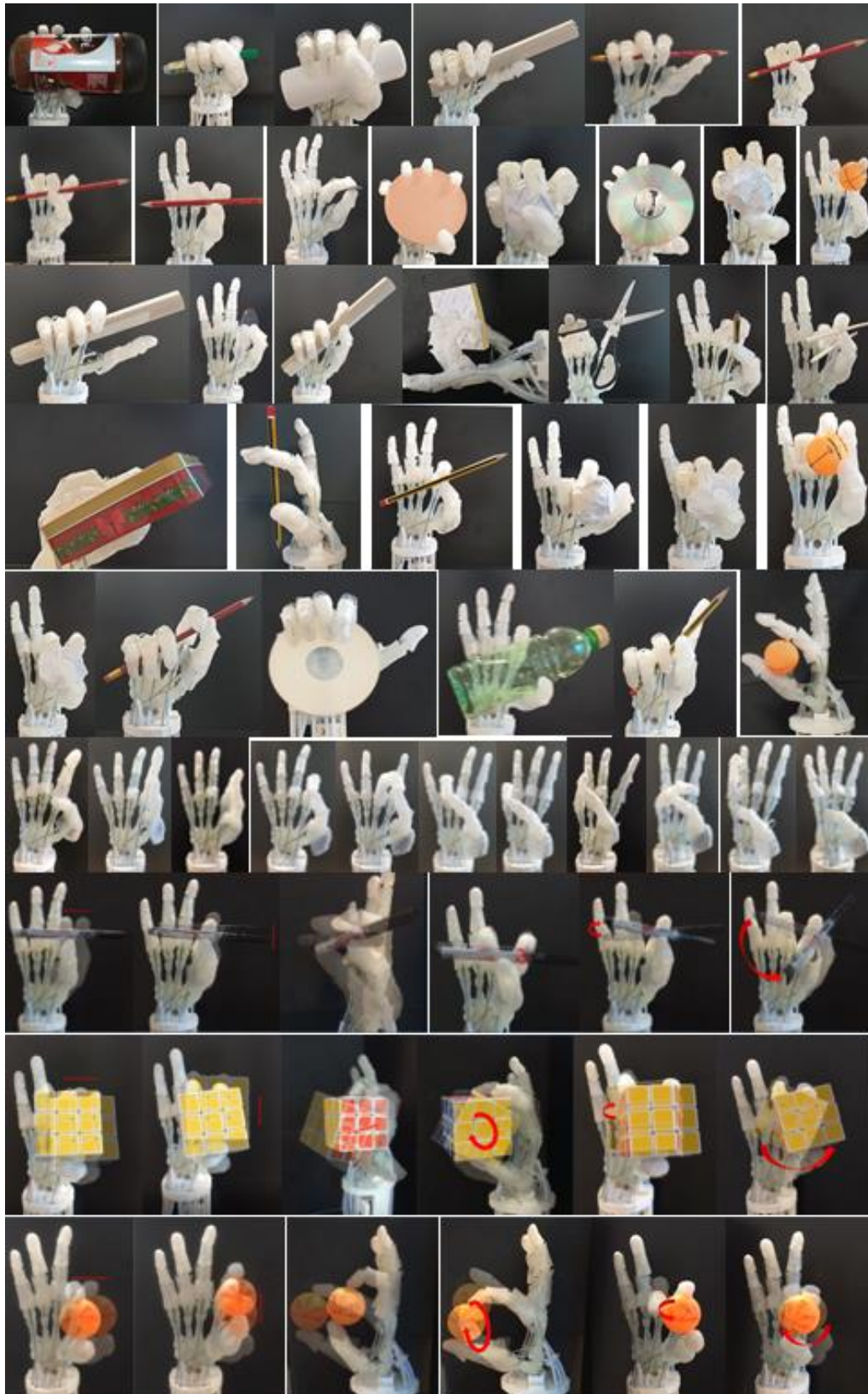
Figure 6-8 Row 1-5 The robotic hand presents the 33 grasping taxonomy tasks. Row 6 presents the achievement of 11 Kapandji tests. Row 7-9 presents translation and rotation cylinder, cuboid and sphere along X, Y and Z-axis.
