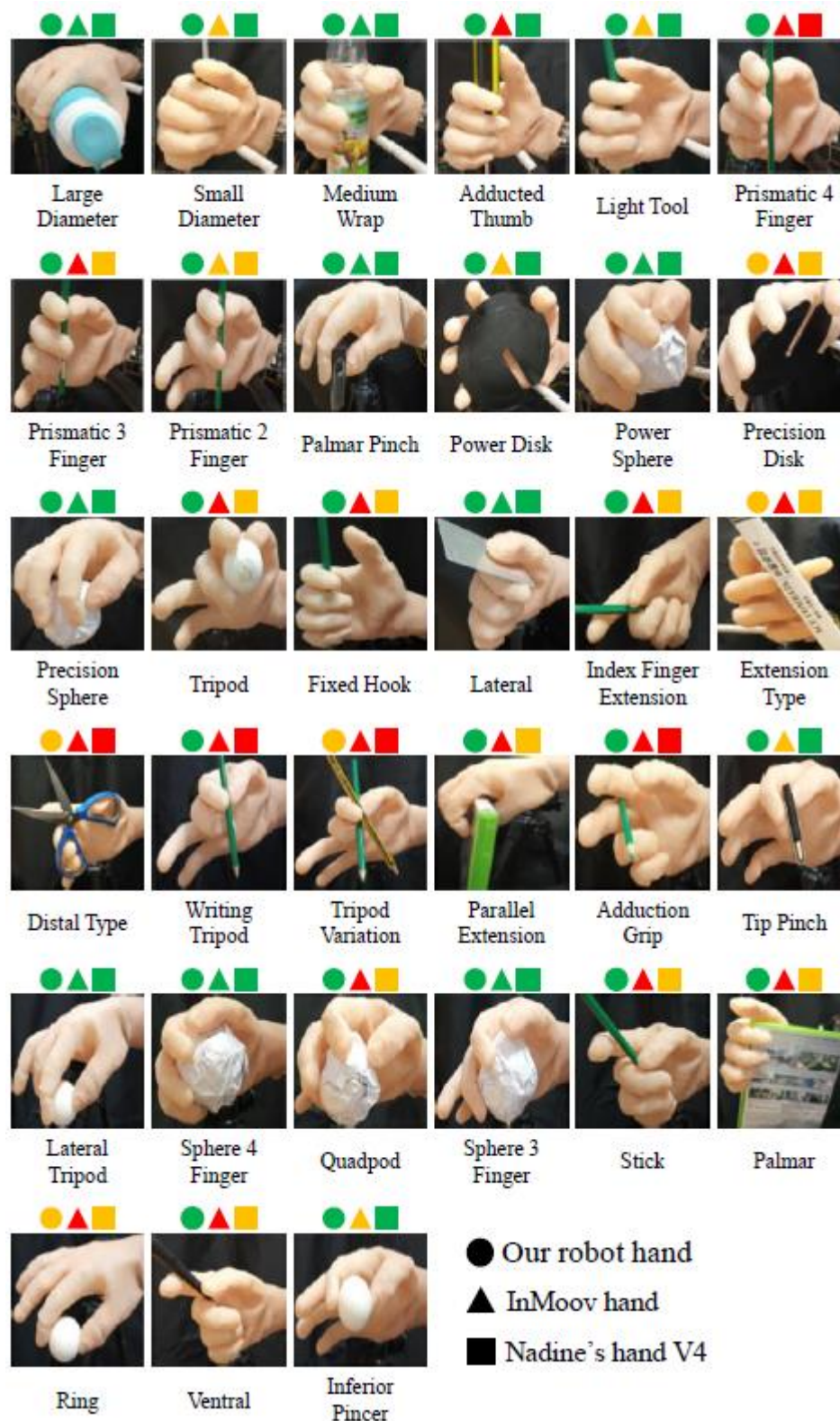
Figure 4-17 Comparison of object grasping success rates of different methods. Methods with success rates \geq 0.8 , in [0.2; 0.8) and < 0.2 are labeled in green, yellow and red, respectively. The proposed robotic hand has the highest success rates for all grasping gestures.
