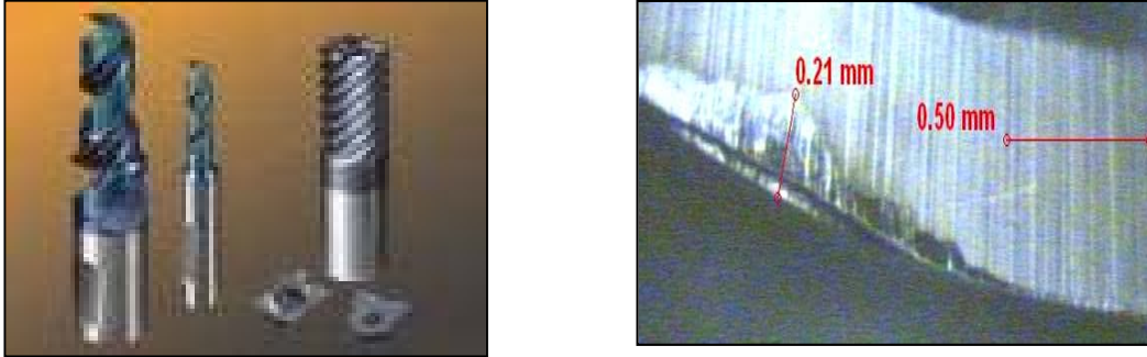
Figure 4.1: Tools and a flank tool wear at cutting edge
