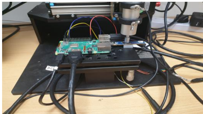
(B) Setup of Raspberry Pi, Probe and NCS2.
