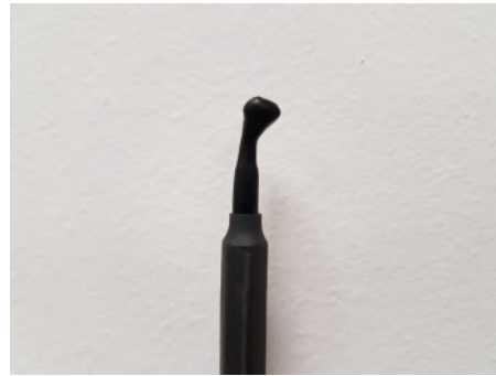
(c) Probe used for measuring EM leakages
