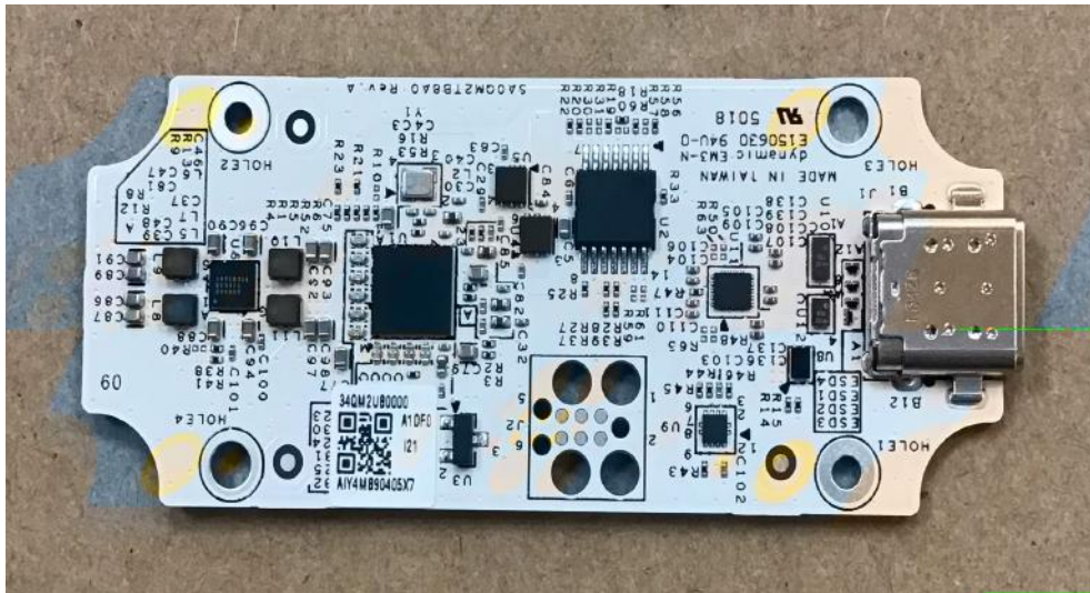
FIGURE 2.8: EdgeTPU Accelerator with its housing and heat sink removed. Attacks are done after removing the housing of the board. This helps to get better reading of the leakages.
