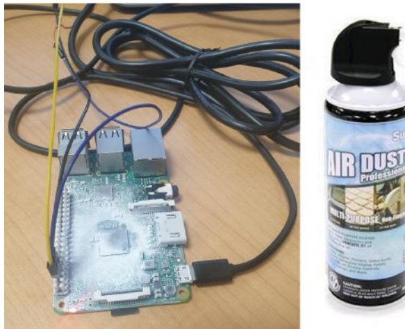
FIGURE 2.9: Raspberry Pi model B+ (Left) frozen using an air duster (Right). Taken from [9]
