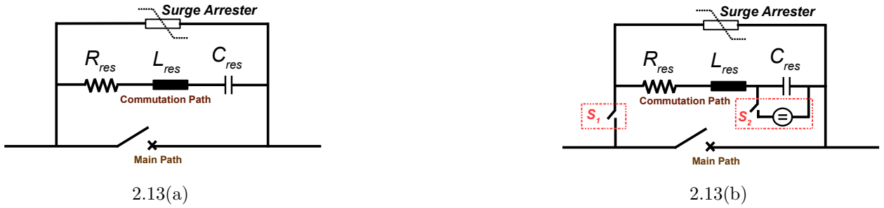
Fig. 2.13: Schematic of dc circuit breaker with (a) passive and (b) active damping.
