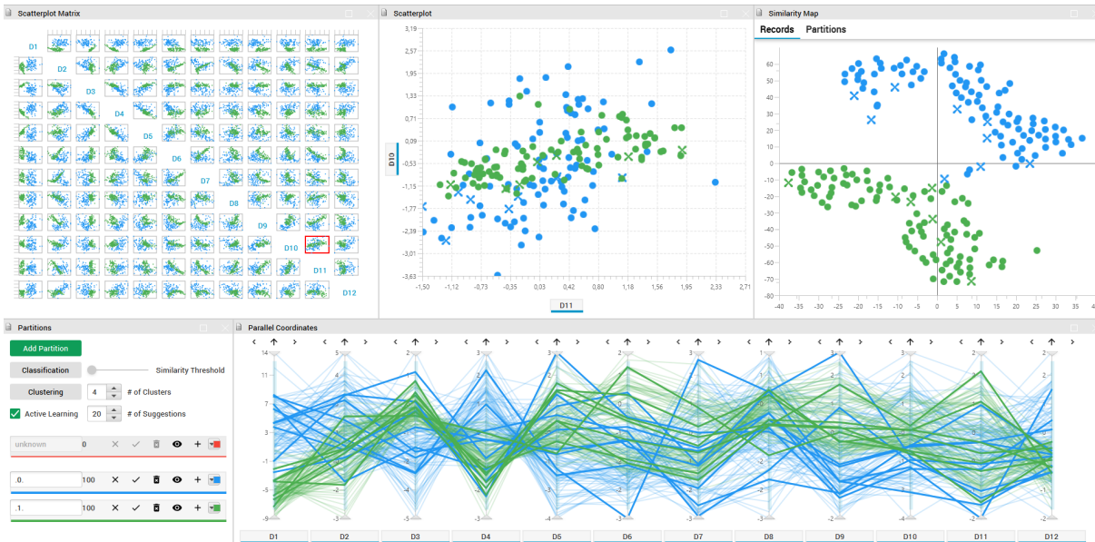
Figure 5.1: The mVis tool, showing the SPLOM at top left, detailed scatterplot top middle, similarity map top right, and parallel coordinates bottom right, for the MNIST2 dataset. The partitions panel at bottom left shows the currently defined classes (label alphabet). Instances are colour-coded by class, here green for 1s and blue for 0s. Instances with confirmed labels are shown as crosses in the scatterplots and similarity map and as thick lines in the parallel coordinates. Suggestions from the classifier are shown as solid circles in the scatterplots and similarity map and as thin lines in the parallel coordinates.
