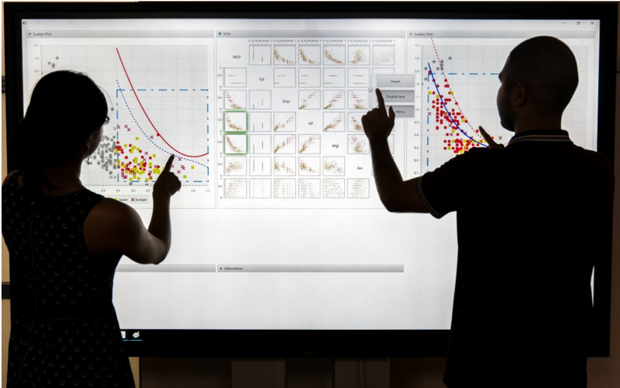
Figure 6.1: Two users collaboratively analyse a dataset on a large vertically-mounted multi-touch screen. User A on the left drags a Regression Lens, while user B on the right adapts the degree of the regression model using the floating toolbox. The display is an Eyevis 84-inch 4K/Ultra-HD 60Hz multi-touch LCD monitor with a resolution of 3840 \times 2160 .
