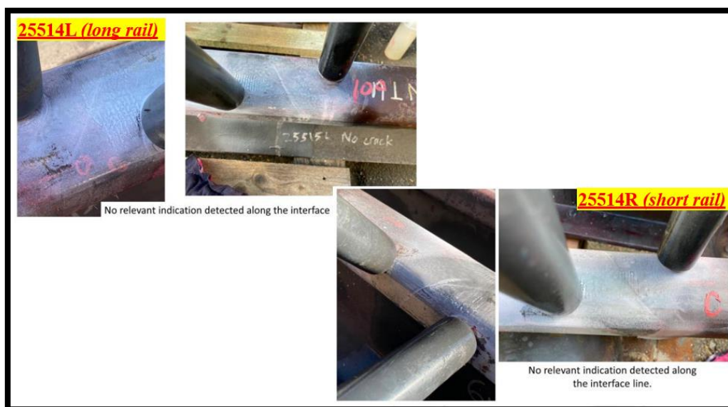
Figure 7-16: MPT Inspection results of extracted specimens 25514L & 25514R
