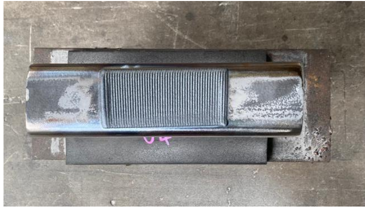
Figure 8-13: SN-1x, refabricated specimen with optimised parameter settings (one layer of Stellite 6 and one layer of Inconel 625)
