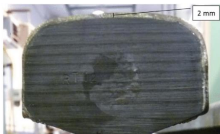
Section of a fully clad R260 60-E2 profile rail to depth of 2mm
