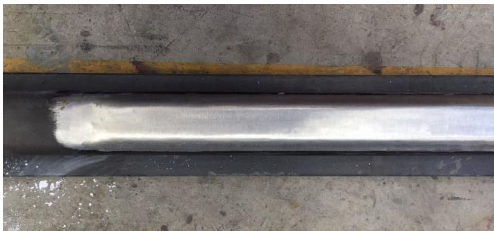
Figure 7-6: Actual clad surface after post grinding
