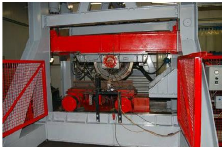
Figure 2-19: Full-scale rail wheel test rig at voestalpine Schienen GmbH [96]
