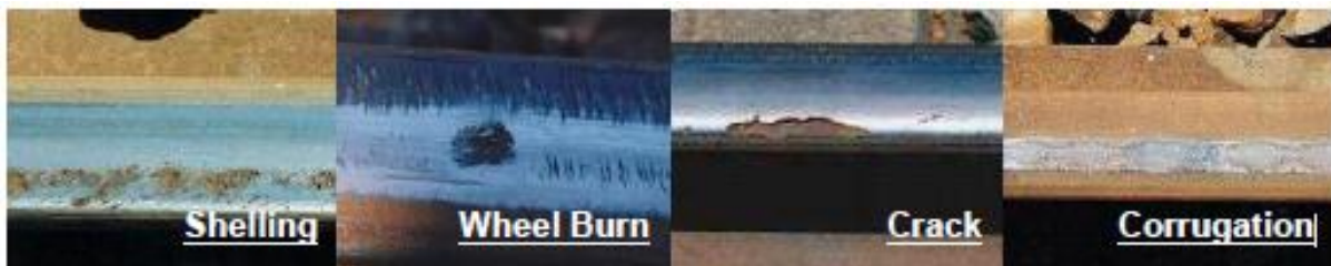
Figure 1-2: Common rail defect types with potential for repair [13]
