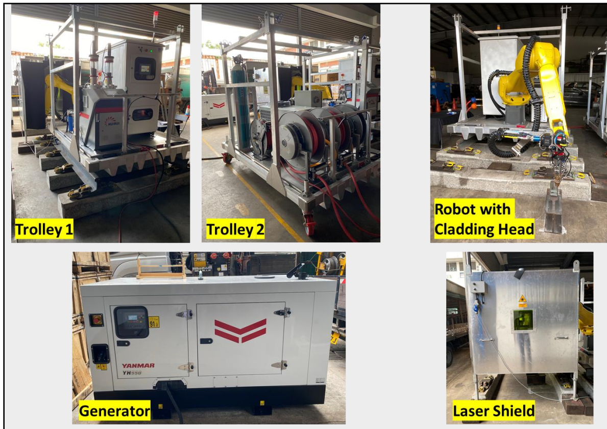
Figure 8-6: Complete setup of the portable laser cladding system
