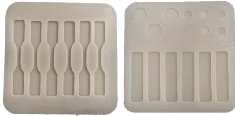
Figure 3.4 Silicone molds with different shape of cavities.
