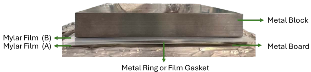
Figure 3.5 The mold setting for preparing disk and film specimens.
