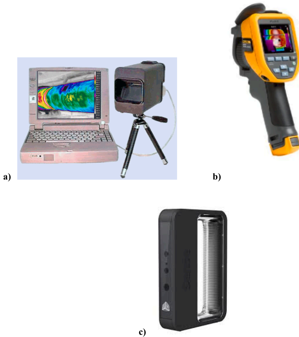
Fig. 4. Equipment used for measurements: a) IRTIS 2000ME; b) Fluke TiS60+ c) 3D Scanner Sense 2.
