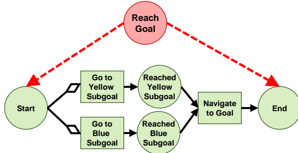
Fig. 3: Concurrent goal pursuit represented by diamond-shaped arcs, indicating that the agent must complete both subgoals before reaching the final goal.
